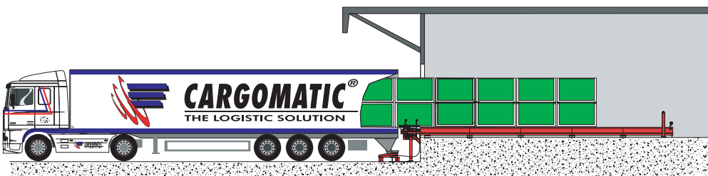
Stationary CM directly on concrete floor, min. height 200 mm.
