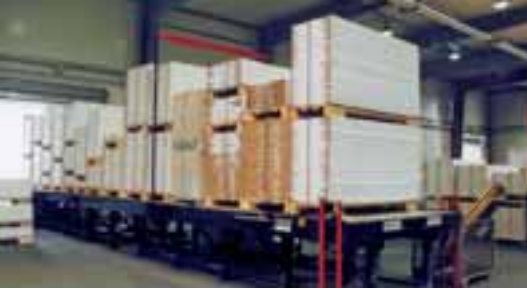
Stationary CM on frame. Height is adjustable using adjustable legs.
