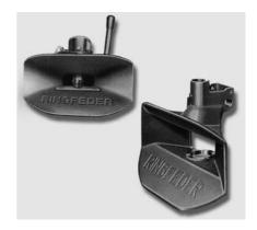
The coupling jaw cannot only be easily locked in the central position, but also in the two lateral end positions; a great advantage when the tractor and trailer have to be coupled in extreme angular positions.
