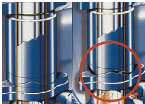
Undulating pressure bearing in the 'straight ahead' position (left) and 'steering' position (right).
